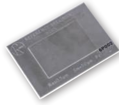
Standard Ra = 0,50 \mu\text{m}
