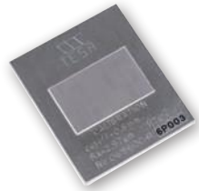
Standard Ra = 2,97 \mu\text{m}
