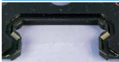
Lip has not been fractured
