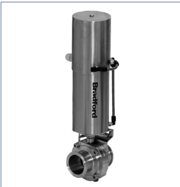
Bradford™ automated butterfly valve with vertical canister air-to-open spring-to-close actuator and control top, with 24VDC solenoid. B5101S200CC-ZB
