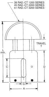
Tensioner body and chain guide width dimensions are same for both standard and compact series, only closed height K/L and guide radii differ.
