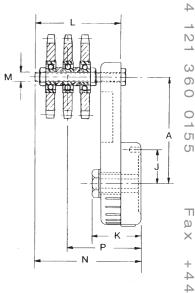
Blind Hole for Location CRT 1000 Series 6mm Ø x 9mm deep CRT 2000 Series 8mm Ø x 9mm deep
