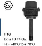
The FT101 sensor is compatible with the API optic or 5 wire signal format. Our probe holder is cast aluminium with a 2" NPT mounting thread, heavy duty stainless steel hardware, and Viton® seals. Install in a 2" NPT female thread or 23/8" hole using the provided gasket and locking nut. (probe housing is part # FT9000).
