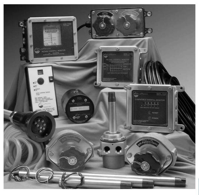
Overfill detection for road tankers is a secondary emergency shut-off system used to prevent overfilling of tanker compartments during the terminal loading process. When an overfill situation is detected, the system will override and shut down the terminal pump/metering equipment filling the tanker compartment(s).
