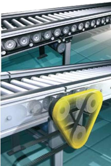
This compact polyurethane synchronous belt opens up new opportunities in the design of conveyor drives and is an alternative to roller chains. Poly Chain® GT Carbon™ does not require lubrication or tensioning and is characterised by low noise levels even at high transport speeds. The special construction is highly resistant to aggressive influences such as dust, oil and chemicals.
