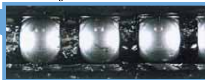
Detail view of the ball cage
