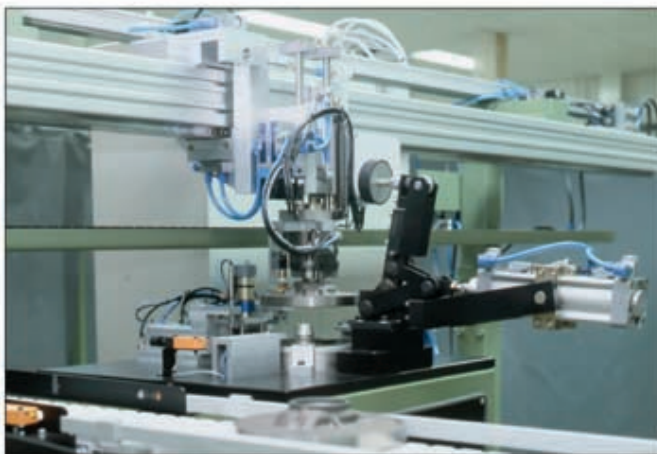
Fully automatic measuring system for pump housing.
