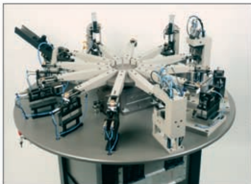
Automatic multistage measuring system for measuring metal parts.
