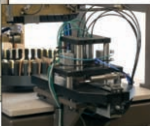
Fully automatic measuring system for measuring the impression depth in linoleum.
