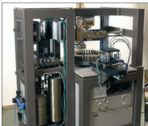
Fully automatic measuring system for measuring the impression depth in linoleum.
