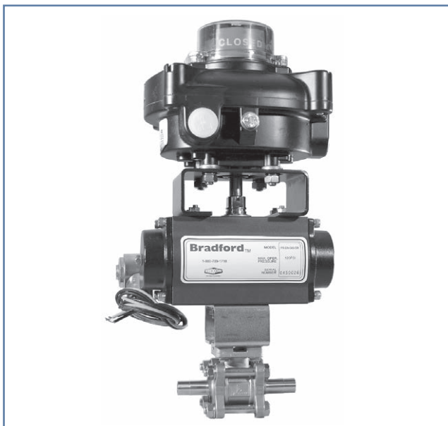
Dixon automated 1/2" encapsulated 2-way ball valve buttweld ends spring return actuator and NEMA 7 (explosion proof) SPDT limit switch with two proximity switches and NEMA 7 NAMUR mount 24VDC voltage solenoid valve pictured. BV2CV-050BB-FPC.
