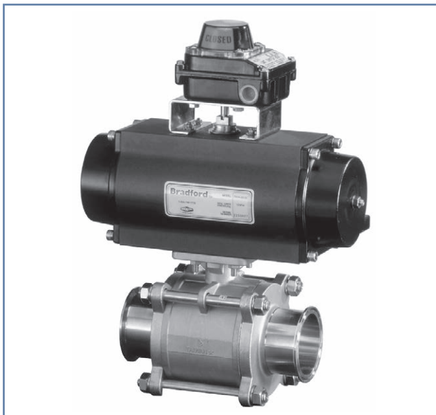
Dixon automated 2 1/2" 2-way encapsulated ball valve with spring return fail close actuator and NEMA 4/4X limit switch with two SPDT mechanical switches pictured. BV2CV-250CC-BFC.
