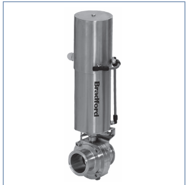
Dixon automated butterfly valve with vertical canister air-to-open spring-to-close actuator and control top, with 24VDC solenoid. B5101S200CC-ZB
