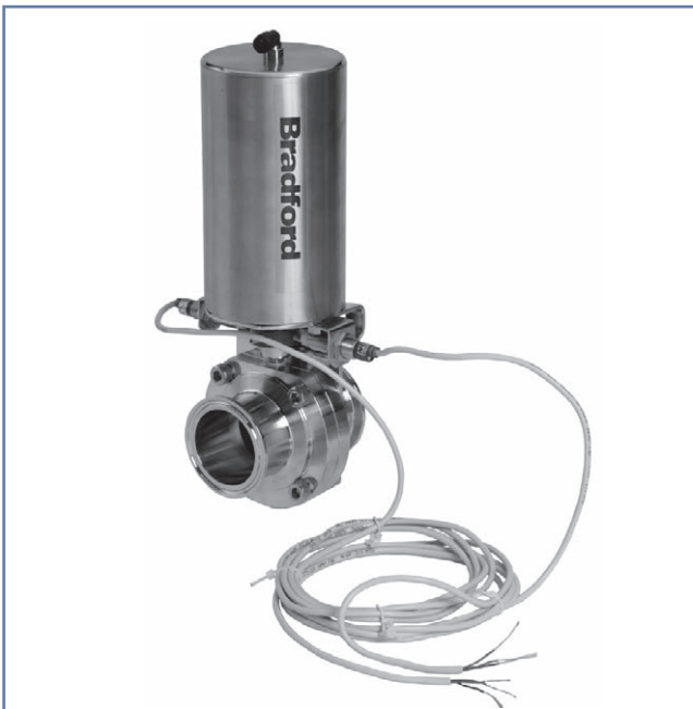
Dixon automated butterfly valve with vertical canister air-to-open spring-to-close actuator and proximity sensors. B5101S200CC-MI
