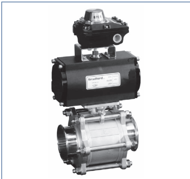
Dixon automated 3" encapsulated ball valve with direct mount double acting, (normally open), actuator and NEMA 7 (explosion proof with 2 mechanical switches) SPDT limit switch pictured. BV2CV-300CC-QAC.
