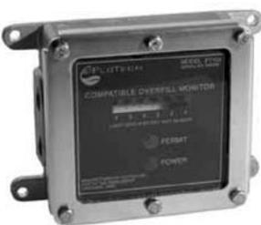
The FT103 API compatible monitor works with the FloTech API compatible sensor models FT101/ 100. This six channel monitor will provide API compatible optic, thermistor, and float socket outputs for a true load at any rack compatibility. Entity approved by CSA and FM to ensure safety. The FT102 replacement chassis is compatible with Civacon 3150 or Scully 08563 on-board monitors.
