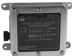
The FT204P retain/overflow monitor is designed to diagnose and monitor up to six compartments. The FT204P monitor will provide API compatible optic, thermistor, and float socket outputs for a true load at any rack compatibility. FloTech's FT203P is a replacement chassis and is compatible with Civacon 3250 and 3252 onboard monitors.
