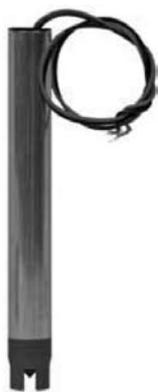
The FT201 is a replacement probe for the FloTech brand FT202 sensor and is compatible with Civacon's 3150 two wire optic probe. The FloTech brand FT200 series probe uses our unique dual elastomer seal prism design to prevent fouling. Other sensor designs use epoxy which crack allowing fuel to leak into the optic path ultimately causing signal malfunction. Custom lengths available upon request (probe housing is part # FT9000).
