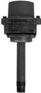
The FT151 thermo-optic sensor contains the FT150 probe and a 2" NPT housing. Our probe holder is cast aluminium with a 2" NPT mounting thread, heavy duty stainless steel hardware, and Viton® probe seal. Install in a 2" NPT female thread or 2 3/8" hole using the gasket and locking nut provided. All screws and rings are heavy duty stainless steel for easy assembly and long life. Compatible with Scully Intellicheck monitors (probe housing is part # FT9000)
