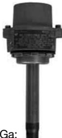
The FT101 sensor is compatible with the API optic or 5 wire signal format. Our probe holder is cast aluminium with a 2" NPT mounting thread, heavy duty stainless steel hardware, and Viton® seals. Install in a 2" NPT female thread or 23/8" hole using the provided gasket and locking nut. (probe housing is part # FT9000).
