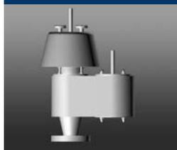
The B100 Series ensures that tanks and vessels are kept safe during periods of excessive pressure and vacuum caused by filling and emptying of product and changes in temperature due to climatic or external fire sources. Available as vent to atmosphere and piped away version.
